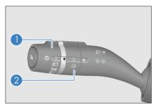
Set the light switch to *B*<sup>□</sup> and push the light switch lever down (away from the steering wheel) to turn on the high beam.
