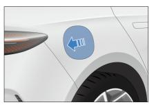
② Open the charge port cap, and make sure that no obstacles exist between the
