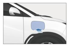
Open the plug cover of the charging gun and the vehicle socket to ensure that there is no obstacle at the end of the charging gun and the charging socket. For AC charging, only the upper charging port plug can be removed, and the lower plug can be kept in a blocked state.
