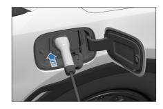
When using the discharging strip, press the switch on the discharging outlet and wait for a few seconds. If the outlet indicator stays on in red, it indicates that the outlet can be used. (Pictures for reference only. The actual local plug standard prevails.)
