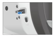
To unlock doors, use the mechanical key to unlock the driver's door first.
