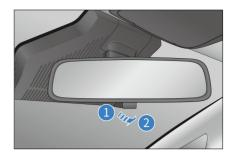
· For nighttime driving - adjusting the control lever to position 2 helps reduce the interference from the cars. behind. Remember that rear view image clarity decreases when glare is reduced.
