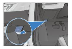
Lift the front hatch cover up and support the front hatch cover with a support rod.
