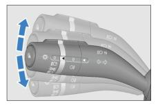
After turn signals are turned on, they flash continuously even if the light switch is released. Turn signals go out automatically after the vehicle finishes turning the corner. Because of different driving habits for drivers, the light switch needs to be rotated for a round to reset in some extreme cases.
