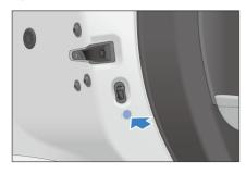
The boot lid opening label is pasted above the opening switch on the right side of the boot lid.
