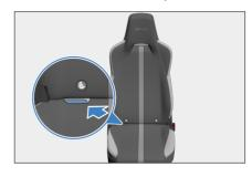
The front passenger seat is equipped with top tether strap anchorages on the back.
