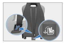
When the child restraint system is installed on the front passenger seat with the top tether, pass it through the hole under the head restraint.
