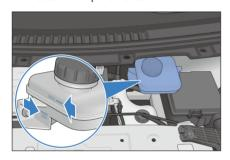
· If the fluid level is at or below the lowest limit (MIN) mark, it is necessary to check the brake system for leakage and wear of brake friction plates.
