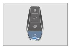
If there is no operation within 10 minutes after remote start, the vehicle stops and powers off, and turn signals flash twice.
