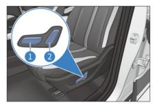
· Push this switch forward or backward to adjust the backrest angle.
