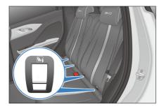
The rear seats are equipped with ISOFIX/i-Size anchorages.
