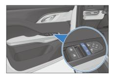
Press the central unlock button to unlock all doors. Once doors are unlocked, the button indicator goes off.
