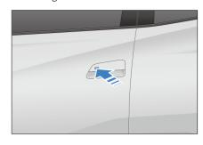
If any door, the hood, or the trunk lid is not closed, pressing the microswitch still locks the closed doors, but the horn only sounds once, and the turn signals do not flash.
